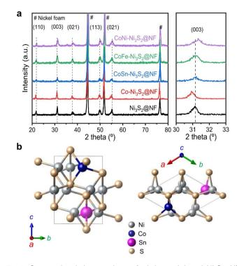
Fig. 1 Structural and phase analyses of pristine and doped-Ni<sub>3</sub>S<sub>2</sub>@NF catalysts using XRD. (a) XRD patterns of Ni<sub>3</sub>S<sub>2</sub>@NF and T-Ni<sub>3</sub>S<sub>2</sub>@NF (T = Co, CoSn, CoFe, and CoNi) catalysts. (b) Heazlewoodite structure of CoSn-Ni<sub>3</sub>S<sub>2</sub> phase with a space group of R32 (155).
