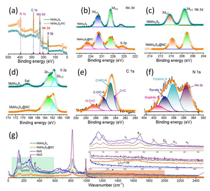
Fig. 2 Structural characterization studies: (a) full scan XPS profiles of NbMo<sub>6</sub>S<sub>8</sub> and NbMo<sub>6</sub>S<sub>8</sub>/NC. Core-level (b) Mo 3d, (c) Nb 3d, and (d) S 2p XPS profiles of NbMo<sub>6</sub>S<sub>8</sub> and NbMo<sub>6</sub>S<sub>8</sub>/NC. Core-level (e) C 1s and (f) N 1s XPS profiles of NbMo<sub>6</sub>S<sub>8</sub>/NC. (g) Raman spectra of NbMo<sub>6</sub>S<sub>8</sub> and NbMo<sub>6</sub>S<sub>8</sub>/NC.
