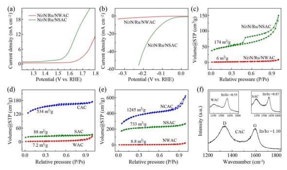
Fig. 4 (a, b) LSV curves of Ni<sub>3</sub>N/Ru/NWAC and Ni<sub>3</sub>N/Ru/NSAC composites for the OER and HER, respectively. Scan rate:  $5 \text{ mV s}^{-1}$ . (c-e) Nitrogen adsorption-desorption isotherms. (c) Ni<sub>3</sub>N/Ru/NWAC and Ni<sub>3</sub>N/Ru/NSAC composites. (d) WACs, SACs and CACs. (e) NWACs, NSACs and NCACs. (f) Raman spectra of WACs, SACs and CACs.
