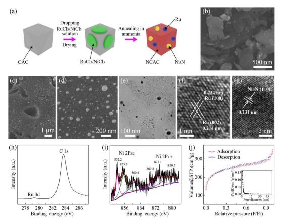
Fig. 1 (a) Schematics of fabrication of Ni<sub>3</sub>N/Ru/NCAC composites. (b) High-magnification SEM image of CACs. (c-e) SEM, high-magnification SEM, and TEM images of Ni<sub>3</sub>N/Ru/NCAC composites, respectively. HRTEM images: (f) Ru and (g) Ni<sub>3</sub>N nanoparticles. High resolution XPS spectra: (h) Ru 3d and (i) Ni 2p. (j) Nitrogen adsorption-desorption isotherm of the Ni<sub>3</sub>N/Ru/NCAC composites. Inset: Pore size distribution curve.
