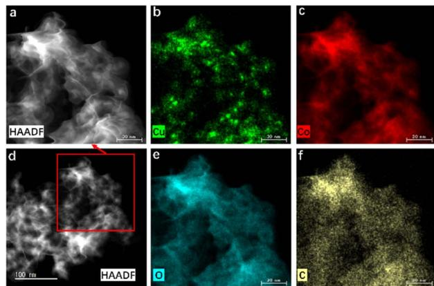
Fig. 3 (a and d) HAADF-STEM images of Cu@CoO<sub>x</sub> derived from Cu-Co-MOF-74 and the corresponding elemental mapping images of (b) Cu, (c) Co, (e) O and (f) C.
