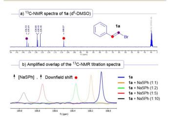
Scheme 4 (a) <sup>13</sup>C-NMR spectra recorded for the compound **1a** in d<sup>6</sup>-DMSO. (b) Overlap of the <sup>13</sup>C-NMR spectra obtained in the titration experiments. Different ratios of the acceptor 1a and electron-donor (NaSPh) were employed to prepare the d<sup>6</sup>-DMSO solutions (from 1:1 to 1:10).
