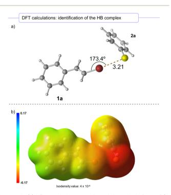
Scheme 5 (a) HB complex between 1a and the anionic form of 2a calculated at the  $\omega B97x$ -D3/Def2TZVPP. (b) Calculated electrostatic potential (red = negative electrostatic potential) on the 0.0004 au isodensity surface.
