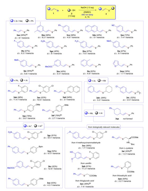
Scheme 2 Substrate scope for the C(sp<sup>2</sup>) – S bond forming photochemical reaction. <sup>a</sup>Also 95% yield when the reaction was run in a 1 mmol scale.  $^b$ K<sub>2</sub>CO<sub>3</sub> as the base (1.5 eq.) and 2.5 h (compounds **3af**, **3an** and **3ja**) and 5 h (compound **3al**) of irradiation time were needed.
