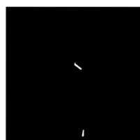
Fig. 3 Deep learning-based micromotor tracking. Simulation and training: (A) Example of a simulated micromotor image generated by DeepTrack 2.1. 33,34 Each image (256 px × 256 px) contains one or more micromotors with aspect ratios similar to those used in the experiments. Bubbles of different sizes (smaller bubbles trailing behind the rods, and larger bubbles in the background) are added to make the images look realistic and thereby closer to the experimental images (see the experimental images in (D) and (G)). For each input image (A), a corresponding output image with a segmentation map (C) is also generated to separate the micromotors from the background and the bubbles. (B) U-Net architecture: A U-Net is employed to transform the input simulated image into the segmentation map. The architectural details and information on each block are indicated in the legend. Inference and analysis: the U-Net model trained on simulated images is then applied on experimental images (D) generating the segmentation maps of the micromotors (E). The positions and orientations of the micromotors are obtained from the segmentation maps. (F) Trajectories: by extracting the positions of all the frames in a video, the trajectories of the micromotors are measured. (G) Each trajectory is further processed to calculate the linear velocities ( v ) and angular velocities ( \omega ). Individual micromotor trajectories are represented in the orange boxes.
