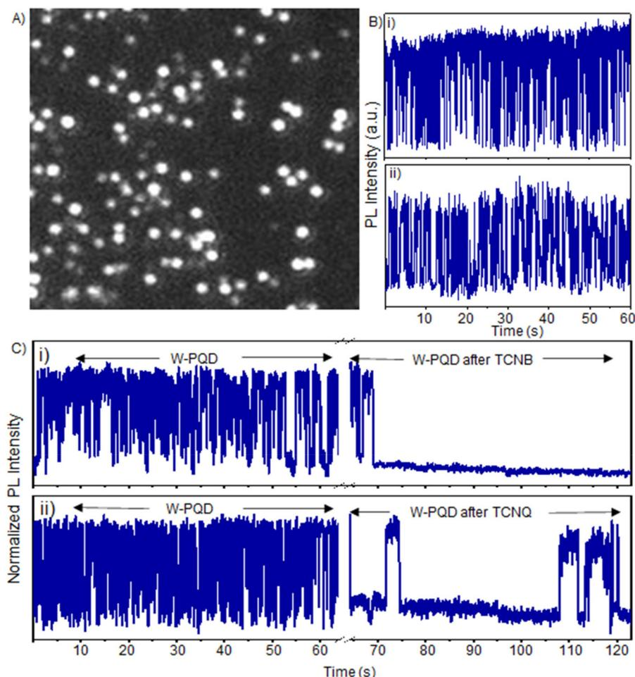
**Fig. 3** PET-induced blinking of single-PQDs. (A) A PL image of W-PQDs on a cover glass substrate and photoexcited at 404 nm ( $585 \text{ W cm}^{-2}$ ). (B) PL intensity trajectories of two pristine W-PQDs. (C) Real-time PL intensity trajectories of single W-PQD immersed in 1-hexadecene (from 0 to 62 s) before and (from 65 to 120 s) after the addition of (i) TCNB (1 mM in toluene) or (ii) TCNQ (1 mM in toluene). The bin size is 33 ms.
