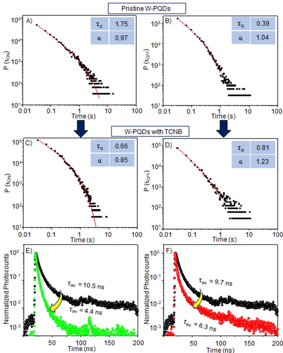
Fig. 4 Blinking time distributions for >400 single PQDs. Probability distributions of (A, C) ON- and (B, D) OFF-times for W-PQDs (A, B) without or (C, D) with TCNB. (E and F) W-PQD's PL decays with or without (E) TCNB and (F) TCNQ. The quencher concentration is 10  $\mu\text{M}$  in both cases.
