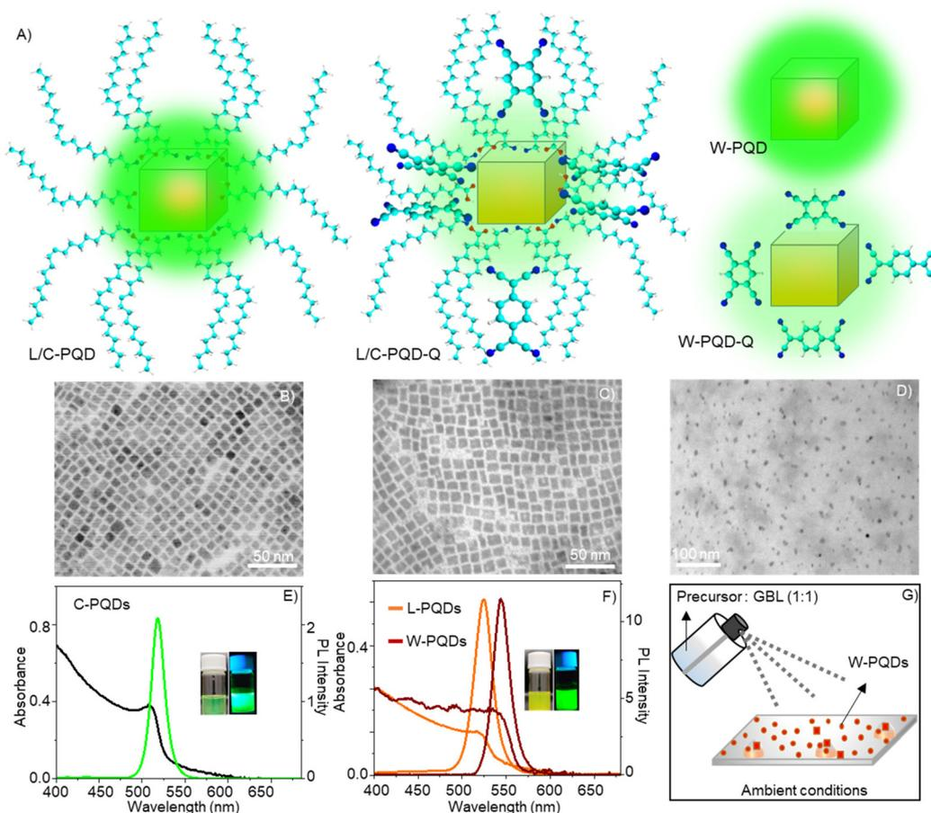
**Fig. 1** Structures and optical properties of PQDs. (A) Schemes of PQDs with or without electron acceptors (quencher, Q = TCNQ/TCNB). (B–D) TEM images of (B) C-PQDs, (C) L-PQDs, and (D) W-PQDs. Absorption and PL spectra of (E) C-PQDs and (F) L-PQDs and W-PQDs (insets: photographs of C/L-PQD solutions taken under room or UV light). The PL spectra were recorded under 400 nm excitation. (G) A scheme of the spray synthesis method.
