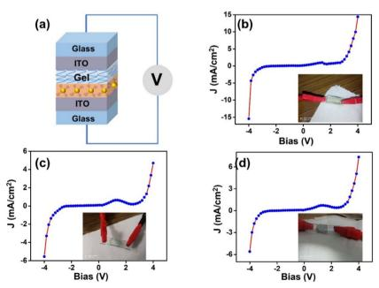
Fig. 6 (a) Schematic representation of device fabrication for I-V measurements, (b)-(d) applied voltage vs. current density plots of Ag NPs, L-Cys@Ag, and D-Cys@Ag NPs, respectively. Inset images show photographs of actual devices.
