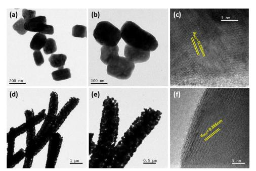
Fig. 4 (a and b) TEM bright field images of hydrothermally synthesized  $WO_3$  nanoparticles at different magnifications, (c) corresponding HRTEM image, (d and e) TEM bright field images of WO<sub>3</sub> fibers synthesized by the electrospinning technique at different magnifications, and (f) corresponding HRTEM image.
