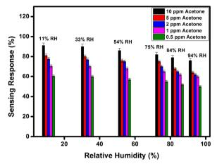
Fig. 8 Sensitivity response bar diagram of the WFS sample as a function of different % RH towards different concentrations of acetone (10, 5, 2, 1 and 0.5 ppm)
