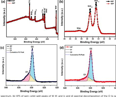
Fig. 2 (a) XPS survey spectrum, (b) XPS of spin-orbit split peaks of W 4f, and (c and d) spectral decomposition of the O 1s spectrum of WF and WP, respectively.
