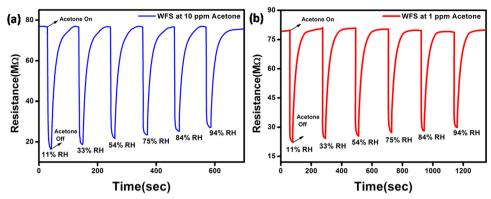
Dynamic response curve of the WFS sensor as a function of different % RH towards (a) 10 ppm and (b) 1 ppm of acetone.
