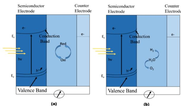
**Fig. 15** Working principle of photoelectrochemical cells. (a) Regenerative-type cell producing electric current from sunlight; (b) a cell that generates a chemical fuel, hydrogen, through the photo-cleavage of water. Reproduced from ref. 212 with permission from Nature Publishing Group UK London, copyright 2001.
