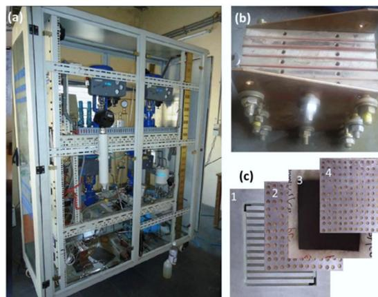
**Fig. 11** (a) Overview of typical PEM water electrolyser, (b) PEM cell stack and, (c) cell components; 1-bipolar plate, 2-anode current collector, 3-MEA, 4-cathode current collector.<sup>181</sup>
