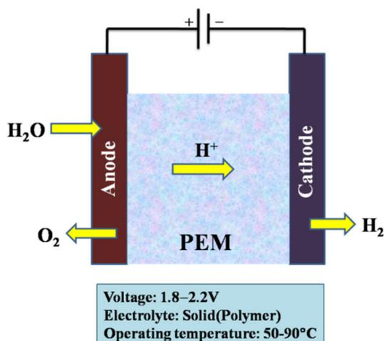
**Fig. 10** Illustration of a PEM electrolysis cell.
