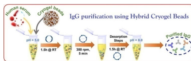
Fig. 24 Use of hybrid alginate-protein cryogel beads to purify IgG (schematic). From ref. 269.
