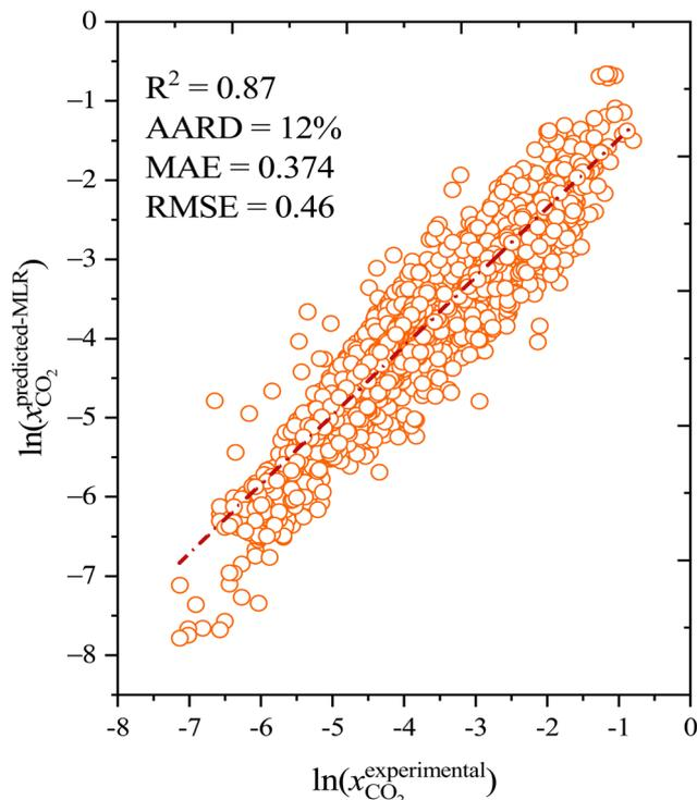
Fig. 5 Correlation between the COSMO-RS corrected multilinear regression model and experimental CO<sub>2</sub> solubility in deep eutectic solvents.
