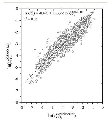
Fig. 4 Correlation between the COSMO-RS predicted and experimental CO<sub>2</sub> solubility in deep eutectic solvents.
