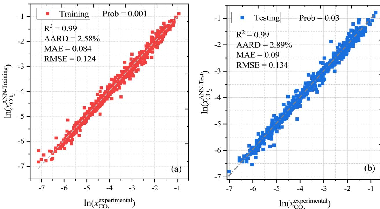
Fig. 6 Experimental and predicted CO<sub>2</sub> solubility in DESs using an ANN-based machine learning model (a) training set and (b) testing set.
