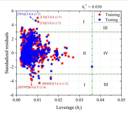
Fig. 8 Williams plot (standardized residual vs. leverage) of the total set of ML model for the CO2 solubility in DESs.
