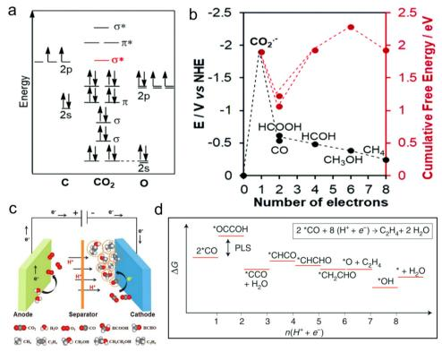
Fig. 6 (a) CO<sub>2</sub> molecular orbital (MO) diagram. (b) Thermodynamic of required activation energy to final product. Reproduced with permission from ref. 111 Copyright 2020, RSC. (c) Design of the cell for the conversion of CO2. Reproduced with permission from ref. 112 Copyright 2018, Wiley. (d) Freeenergy diagram with favourable reaction path for CO<sub>2</sub> to C<sub>2</sub>H<sub>4</sub> on Cu surface. Reproduced with permission from ref. 65 Copyright 2019, Springer Nature.
