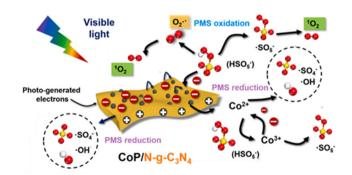
Fig. 6 The proposed mechanism in the CoP/N-g-C<sub>3</sub>N<sub>4</sub> nanosheets catalyzed visible-light-driven PMS activation. Copied with permission from ref. 33. Copyright 2021, Elsevier.
