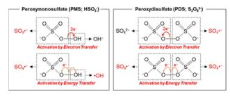
Fig. 5 Activation of PMS and PDS via electron- and energy-transferring processes. Copied with permission from ref. 91. Copyright 2020, American Chemical Society
