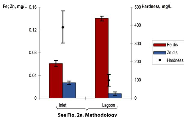
**Fig. 7** Metals and water hardness profile during dry weather Fe<sub>dis</sub> is 0.14 mg L<sup>-1</sup> in the lagoon, comprising almost 50% of its total form (Fe<sub>tot</sub> is 0.29 mg L<sup>-1</sup>).
