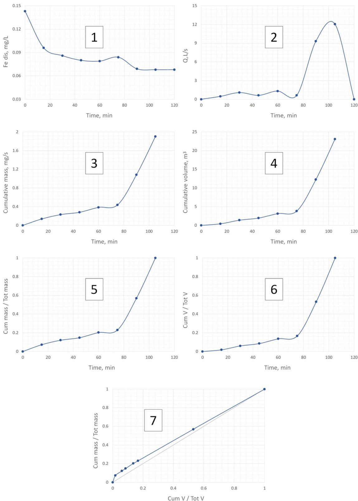
Fig. 5 Example of the drawing of one  $M(V)$  curve for  $Fe_{dis}$  for event 2. The numbers 1–7 indicate the order of drawing each point of the  $M(V)$  curve from both the hydrograph and the pollutograph.
