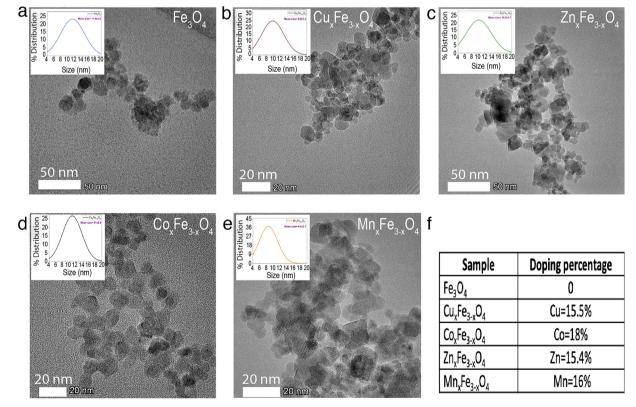
Fig. 2 TEM images showing the morphology and particle size distribution (shown in inset) of (a)  $Fe_3O_4$  (b)  $Cu_xFe_{3-x}O_4$  (c)  $Co_xFe_{3-x}O_4$  (d)  $Zn_xFe_{3-x}O_4$  (e)  $Mn_xFe_{3-x}O_{4r}$  (f) dopant concentration in ferrites as measured by ICP-MS.
