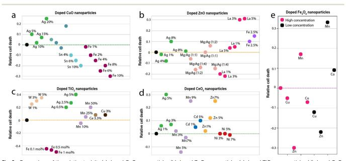
Fig. 8 Comparison of the relative toxicity (a) doped CuO nanoparticles (b) doped ZnO nanoparticles (c) doped TiO<sub>2</sub> nanoparticles (d) doped CeO<sub>2</sub> nanoparticles and (e) doped ferrite nanoparticles. The dotted line in each case is the baseline (the toxicity of the undoped nanoparticle). The data and references used to generate these graphs is reported in the ESI.†
