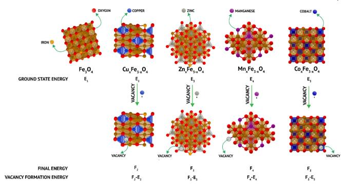
Fig. 1 Schematic of density functional theory (DFT) calculations of the vacancy formation energy in doped and undoped ferrites.
