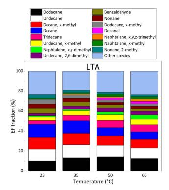
Fig. 7 Evolution of VOC emission composition in % for the species accounting for more than 75% of VOC emissions (EF > 3.63  $\mu$ g m<sup>-2</sup> h<sup>-1</sup> for LTA asphalt mixtures) as a function of temperature, as measured by GC-MS/FID under dry (RH = 0.1%) and dark conditions, for the LTA2 old asphalt sample.
