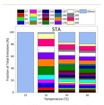
Fig. 4 Evolution of VOC emission composition in % for the 20 masses exhibiting the strongest contributions (EF > 22  $\mu g$  m $^{-2}$  h $^{-1}$  at 60 °C) as a function of temperature, as measured by PTR-ToFMS under dry (RH = 0.1%) and dark conditions, for the STA3 fresh asphalt sample.
