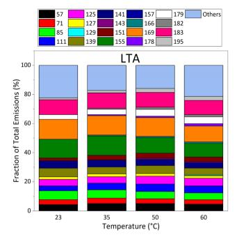
Fig. 5 Evolution of VOC emission composition in % for the 20 masses exhibiting the strongest contributions (EF > 22  $\mu$ g m<sup>-2</sup> h<sup>-1</sup> at 60 °C) as a function of temperature, as measured by PTR-ToFMS under dry (RH = 0.1%) and dark conditions, for the LTA2 old asphalt sample.
