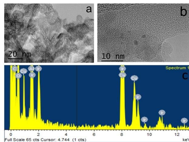
Fig. 9 A and B. HRTEM images of 3@Al<sub>2</sub>O<sub>3</sub>-uncal after 45 h reaction at 350 °C with  $0.10 \text{ mL min}^{-1}$  flow rate. A few particles, 2–3 nm in diameter are visible at higher magnification. The lattice spacing corresponds to metallic Ir. C. XEDS spectra of 3@Al<sub>2</sub>O<sub>3</sub>-uncal after 45 h reaction.
