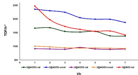
Fig. 4 Reactivity of different catalysts at 325 °C at 0.09 mL min<sup>-1</sup> flow rate.
