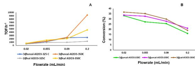
Fig. 8 A) Initial TOF ( $\text{h}^{-1}$ ) at different flow rates, obtained using 2@Al<sub>2</sub>O<sub>3</sub>-cal-325 °C, 3@Al<sub>2</sub>O<sub>3</sub>-cal-350 °C, 3@Al<sub>2</sub>O<sub>3</sub>-uncal-325 °C and 3@Al<sub>2</sub>O<sub>3</sub>-uncal-350 °C (left). B) Initial conversion (%) at different flow rates, obtained using 3@Al<sub>2</sub>O<sub>3</sub>-cal-350 °C, 3@Al<sub>2</sub>O<sub>3</sub>-uncal-325 °C and 3@Al<sub>2</sub>O<sub>3</sub>-uncal-350 °C (right).
