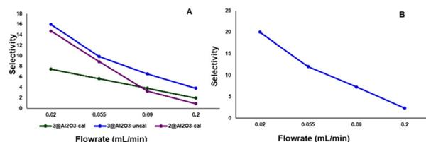
Fig. 7 A) Selectivity for P3 at different flow rates, obtained using 2@Al<sub>2</sub>O<sub>3</sub>-cal, 3@Al<sub>2</sub>O<sub>3</sub>-cal and 3@Al<sub>2</sub>O<sub>3</sub>-uncal at 325 °C (left). B) Selectivity for P3 at different flow rates obtained using 3@Al<sub>2</sub>O<sub>3</sub>-uncal at 350 °C (right).
