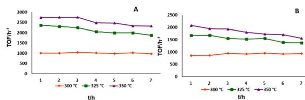
Fig. 5 Reactivity of **3@Al<sub>2</sub>O<sub>3</sub>-uncal** (A) and **3@Al<sub>2</sub>O<sub>3</sub>-cal** (B) at 300 °C, 325 °C and 350 °C.
