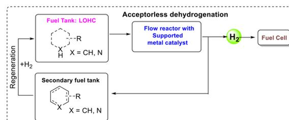
Fig. 1 Concept of LOHCs under continuous-flow conditions.
