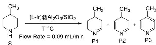
Scheme 4 Dehydrogenation of 4-methylpiperidine with different catalysts.
