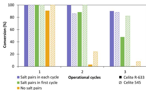
**Fig. 5** Influence of salt pairs on the reduction of cyclohexenone **1a** catalysed by immobilised *TsOYE* in MTBE. Conditions: 10 mmol **1a**, 1 mmol NADP<sup>+</sup>, 2 mg GDH-101, 27.7 mmol glucose, 25 mg Na<sub>2</sub>HPO<sub>4</sub>·12H<sub>2</sub>O/Na<sub>2</sub>HPO<sub>3</sub>·5H<sub>2</sub>O or no salt pairs (yellow), 50 mg *TsOYE*-Celite R-633 (full pattern) or 545 (stripped pattern), MTBE (2% v/v buffer content), 1 mL volume, 900 rpm, 30 °C, 24 h.
