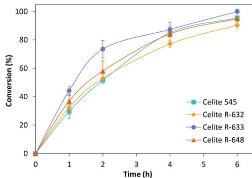
**Fig. 3** Reduction of cyclohexenone **1a** catalysed by immobilised *TsOYE* in MTBE. Conditions: 50 mg *TsOYE*-Celite, 10 mmol **1a**, 1 mmol NADP<sup>+</sup>, 27.7 mmol glucose, 25 mg Na<sub>2</sub>HPO<sub>4</sub>·12H<sub>2</sub>O/Na<sub>2</sub>HPO<sub>3</sub>·5H<sub>2</sub>O, 2 mg GDH-101, MTBE, 1 mL volume, 900 rpm, 30 °C.
