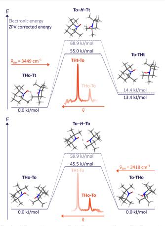
Fig. 4 HAT transition states T-H-T between different TH-T complex arrangements at B3LYP/TZ level, including and excluding zero point energy correction. The excitation wavenumber for OH stretching obtained from experiment is also indicated. A non-degenerate path segment for THo-Tt (upper) and the degenerate path for THo-To (lower panel) is explored. Slightly different values obtained with ORCA 5.0.3 can be found in the ESI.†
