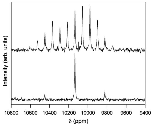
Fig. 12  $^1\text{H}$ - $^{103}\text{Rh}$  CP-MAS NMR spectra of  $[(\text{H}_2\text{O})_4\text{Rh}(\mu_2\text{-OH})_2\text{Rh}(\text{H}_2\text{O})_4](\text{dmtos})_4 \cdot 8\text{H}_2\text{O}$  comparing spinning rates of 1.0 (top) and 4.0 kHz (bottom). Both spectra acquired with 8 ms contact time, 5 s relaxation delay for 12 000 (top) and 15 800 (bottom) acquisitions.<sup>37</sup> Reproduced from the ref. 37 with permission from the American Chemical Society, copyright 2006.
