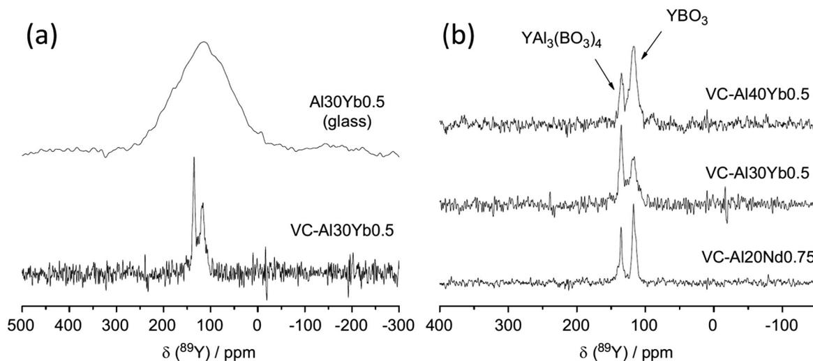
**Fig. 10** Application of  $^{89}\text{Y}$  MAS NMR to probe glass to ceramic transitions, with an example given for (a)  $(\text{Y}_2\text{O}_3)_{0.1}(\text{Al}_2\text{O}_3)_{0.3}(\text{B}_2\text{O}_3)_{0.6}$  ( $\text{Al}_3\text{O}$ ) Yb-doped sample and (b) comparison of the major yttrium phases that form for different aluminium levels as well as a comparison of ytterbium to neodymium.<sup>105</sup> Reproduced from ref. 105 with permission from Elsevier, copyright 2012.
