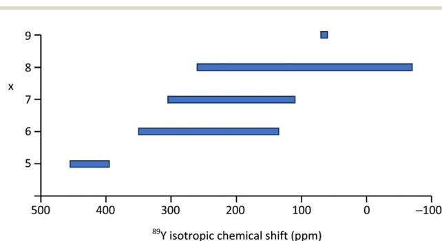
Fig. 8  $^{89}\text{Y}$  isotropic chemical shift ranges associated with  $\text{YO}_x$  local coordinations based on the values reported in the literature as given in Table 2 or summarised previously.<sup>2,5</sup>
