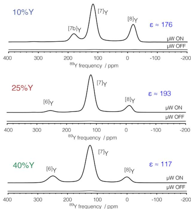
**Fig. 3**  $^{89}\text{Y}$  MAS NMR Hahn-echo spectra from co-precipitated ceria samples with various levels (10, 25 and 40%) of  $\text{Y}_2\text{O}_3$  substitution and 0.1%  $\text{Gd}_2\text{O}_3$  showing the signal enhancement ( $\epsilon$ ) *via* DNP when microwaves ( $\mu\text{W}$ ) are applied, with the different yttrium coordinations  $^{[x]}\text{Y}$  observed.<sup>53</sup> Reproduced from ref. 53 with permission from the American Chemical Society, copyright 2021.
