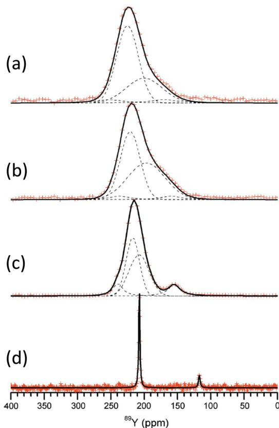
Fig. 9  $^{89}\text{Y}$  CPMG MAS NMR spectra of  $\text{Y}_x\text{Sc}_{2-x}\text{Si}_2\text{O}_7$  with (a)  $x = 0.5$ , (b) 1.0, (c) 1.5 and (d) 2.0. As scandium is added the appearance of more lines suggests inequivalent sites result from differing NNN yttrium and scandium.<sup>100</sup> Reproduced from ref. 100 with permission from the International Union of Crystallography, copyright 2011.
