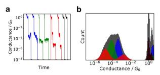
Fig. 4 (a) Typical conductance traces and (b) conductance histograms of simulated data. The dataset is constructed from four classes with 1000 traces. Black, blue, red, and green histograms represent histograms of each class. Gray histogram the cumulative histogram of all data. Gray histogram cannot provide conductance information of each state.
