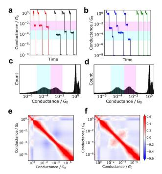
Fig. 3 Examples of 2DCH. Two datasets constructed from 1500 simulated data were analysed. (a and b) Typical conductance traces. (c and d) Conductance histograms (e and f) 2D correlation histograms. (a, c and e) and (b, d and f) were obtained from each dataset
