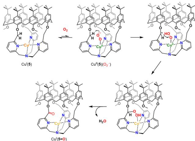
Fig. 6 Proposed mechanism for intramolecular C–H bond oxidation upon O<sub>2</sub> activation in Cu<sup>I</sup>(**5**). A similar pathway is proposed for Cu<sup>I</sup>(**4**).
