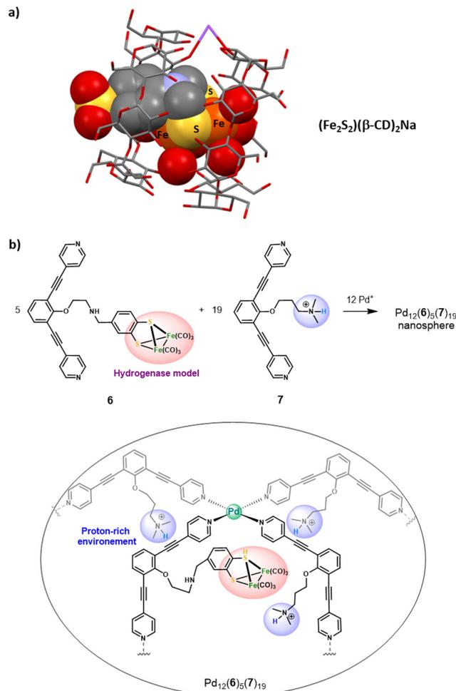
Fig. 7 (a) Representation of the XRD structure of (Fe<sub>2</sub>S<sub>2</sub>)(β-CD)<sub>2</sub>Na. (b) Confinement of five hydrogenase mimicking clusters in a proton rich the Pd<sub>12</sub>(**6**)<sub>5</sub>(**7**)<sub>19</sub> nanosphere (top), along with the schematic representation of one of the five catalytic centers found in the nanosphere (bottom).
