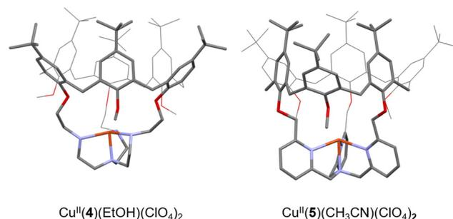
Fig. 5 Views of the XRD structures of Cu<sup>I</sup> complexes based on the **4** and **5** calix[6]arene-based ligands. Counter ions and bounded molecules of solvent (EtOH and CH<sub>3</sub>CN, respectively) have been omitted for clarity.
