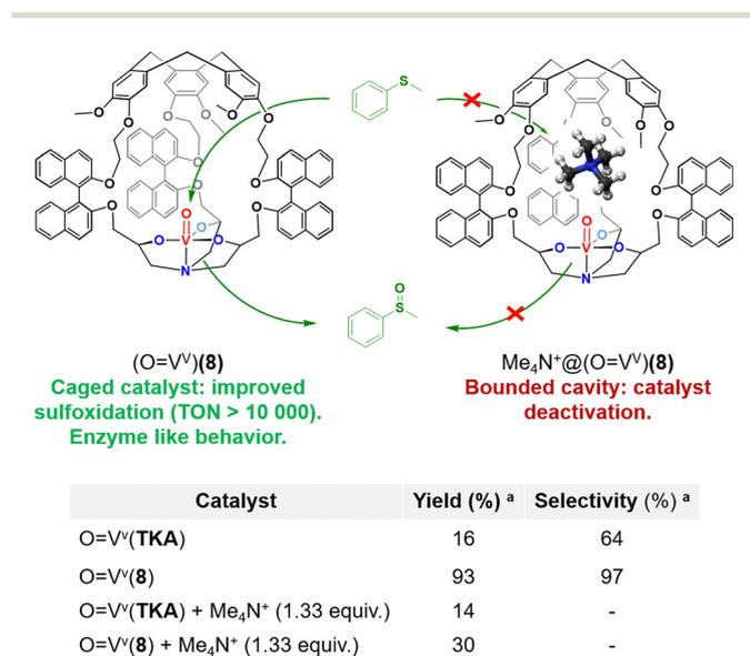
Fig. 8 (Top) Representation of the efficient sulfoxidation observed in caged oxido-vanadium catalyst ( $O=V^V$ )(**8**) (left), and catalyst inhibition observed upon tetramethylammonium binding in the catalyst cavity (right). (Bottom) Comparison with its open analogue devoid of the CTV cap ( $O=V^V$ )(TKA).<sup>a</sup>Oxidation of thioanisol in the presence of the catalyst (1.5 mol%) and CHP (1.0 equiv.) for 180 min in  $CH_2Cl_2$  at 0 °C.
