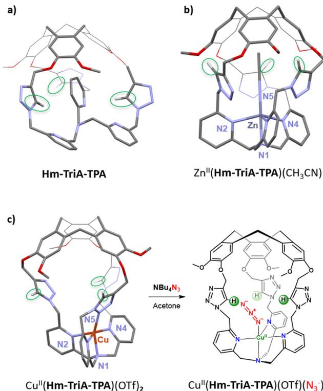
Fig. 12 Views of the DFT structures of (a) the cage-ligand **Hm-TriA-TPA** and (b) its corresponding  $\text{Zn}^{\text{II}}$  complex. (c) View of the XRD structure of  $\text{Cu}^{\text{II}}(\text{Hm-TriA-TPA})(\text{OTf})_2$  along with formation of the corresponding azido adduct upon addition of tetrabutylammonium azide.
