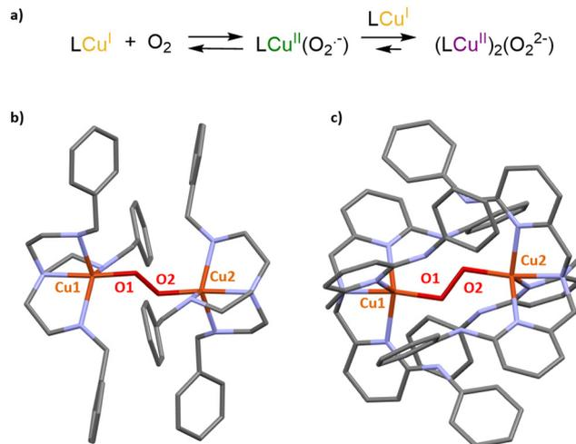
Fig. 4 (a) Formation of primary and secondary O<sub>2</sub> adducts arising from O<sub>2</sub> activation in open Cu(I) complexes. XRD structures of [(Cu(L))<sub>2</sub>(O<sub>2</sub>)] peroxo dimers observed upon O<sub>2</sub> activation in (b) Cu<sup>I</sup>(TREN) and (c) Cu<sup>I</sup>(TPA) derivatives.
