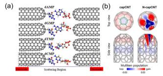
Fig. 6 (a) Atomic structure of the functionalized closed-end cap CNTbased nanogap setup for the detection of four different nucleotides (dAMP, dGMP, dTMP, and dCMP). The CNT electrodes (left and right) are semi-infinite and periodic along the transport direction (z-axis). 196 (b) Charge distributions in the pristine and N-doped capped CNTs.  $^{197}$ Figures adapted with permission from the American Chemical Society, Copyright (2018) and The Royal Society of Chemistry, Copyright (2020).
