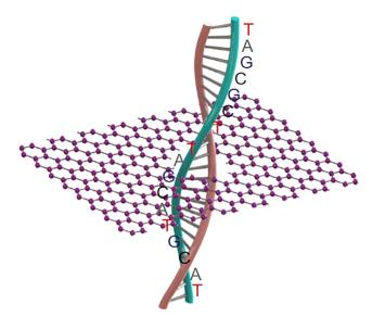
Fig. 1 Schematic DNA sequencing through a carbon nanopore.
