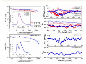
Fig. 4 (a) EQE-luminance curves of the green CP-OLED devices (inset: normalized EL spectra); (b) CPEL spectra and  $g_{\rm EL}$  values of the devices versus wavelength curves; (c) EQE-luminance curves of the CP-OLED with two emitters (inset: normalized EL spectra) and (d) CPEL spectra and  $g_{\rm EL}$  values of the CP-OLED with two emitters versus wavelength curves.
