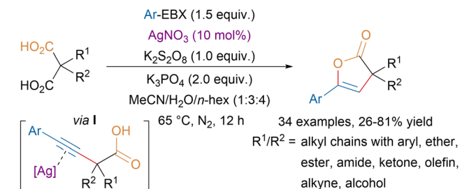
Scheme 34 Ag-catalyzed monodecarboxylative alkynylation–lactonization of malonic acid derivatives.
