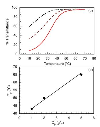
Fig. 2 (a) Percent transmittance (%T) of EUM in PBS at various  $C_p = 1.0$ (----), 2.0 (----), and 5.0 g  $L^{-1}$  (-----) as a function of temperature with the cooling process, and (b) phase transition temperature ( $T_p$ ) of EUM in PBS as a function of  $C_p$ .
