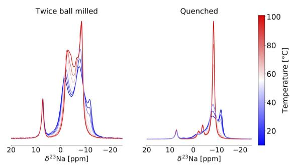
Fig. 9 23Na variable temperature ss-NMR spectra collected on the twice ball milled (left) and quenched (right) Na<sub>2.25</sub>Y<sub>0.25</sub>Zr<sub>0.75</sub>Cl<sub>6</sub> samples. Spectra are color-coded using the temperature scale to the right of the plots. The resonance at 7.2 ppm corresponds to NaCl. All spectra were obtained at 18.8 T and at a 10 kHz MAS speed.
