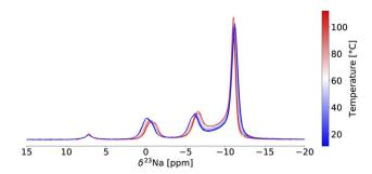
Fig. 3 Variable temperature  $^{23}$ Na ss-NMR on twice ball milled Na<sub>2</sub>-ZrCl<sub>6</sub>. Spectra are color-coded using the temperature scale on the right of the plot. The peak at 7.2 ppm is NaCl. All spectra were obtained at 18.8 T with a 10 kHz MAS speed.
