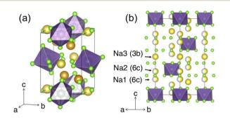
Fig. 4 Polymorphs of the Na<sub>3</sub>YCl<sub>6</sub> composition. Color legend: Y is purple, Cl is light green, while Na atoms in octahedral and prismatic environments are yellow and orange, respectively. (a) The  $P2_1/n$ structure with Na occupying prismatic and octahedral sites. (b) The  $R\bar{3}$ polymorph, as seen down the [110] direction. The three Na sites are depicted with varying degrees of occupancy, as reported by Stenzel and Meyer.29
