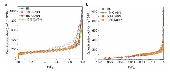
N<sub>2</sub> sorption isotherms at 77 K for BN samples in (a) linear scale; (b) semi-log scale. Filled symbols: adsorption. Empty symbols: desorption.
