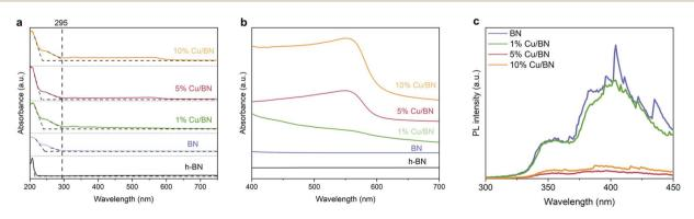
Optoelectronic properties Cu/BN with different Cu contents. (a) DRS UV-vis absorption spectra compared to that of hBN; (b) zoom of the panel (a) spectra in the range of 400-700 nm wavelength; (c) PL spectra obtained using a 250 nm excitation wavelength.
