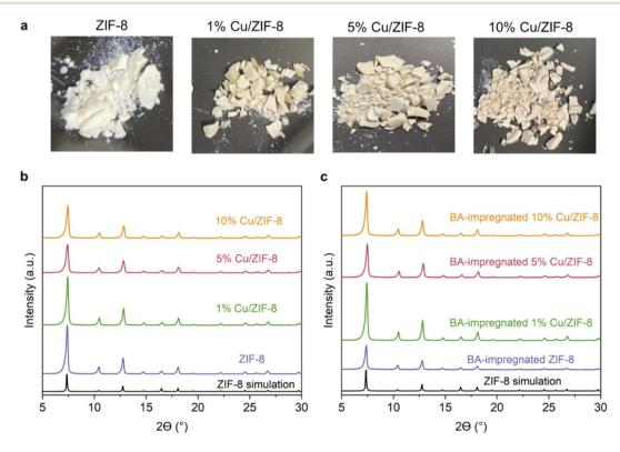
Fig. 1 Appearance and structural features of ZIF-8 and Cu/ZIF-8 samples: (a) optical images; (b) XRD patterns; (c) XRD patterns of BAimpregnated Cu/ZIF-8 samples.
