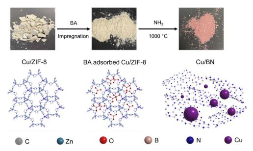
Scheme 1 Schematic representation of Cu/BN synthesis
