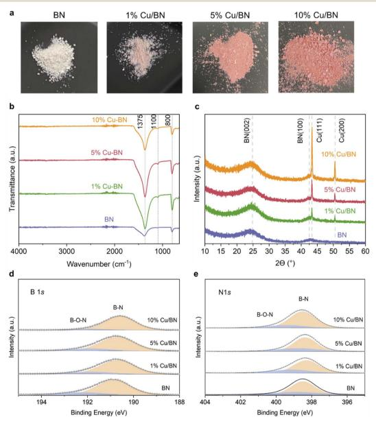
Fig. 2 Appearance, structural features and chemical features of BN and Cu/BN samples with varying Cu contents: (a) optical images; (b) FTIR spectra; (c) XRD patterns; (d) high resolution XPS and peak fittings of the B 1s core level; (e) high resolution XPS and peak fittings of the N 1s core level.
