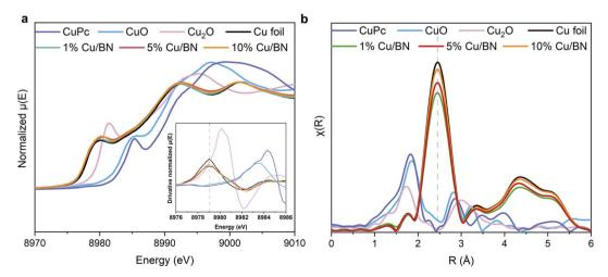
Fig. 3 XAS characterisation of Cu/BN samples with varying Cu contents and reference samples. (a) Normalised Cu K-edge XANES spectra; inset: derivative Cu K-edge spectra; (b) phase corrected  $k^2$ -weighted Fourier transformed EXAFS spectra, using k-range 3-11 Å<sup>-1</sup>.
