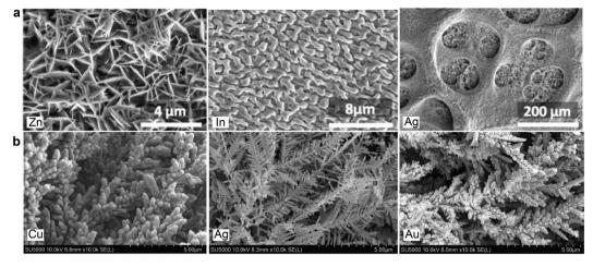
**Fig. 9** Scanning electron micrographs of (a) porous Zn, In, and Ag electrodes prepared by hydrogen-bubble-templated electrodeposition technique, reproduced with permission, <sup>60</sup> copyright 2017, John Wiley and Sons. (b) Cu, Ag, and Au nano dendrites on glassy carbon prepared *via* galvanic replacement reaction. Reproduced with permission, <sup>74</sup> copyright 2020, John Wiley and Sons.
