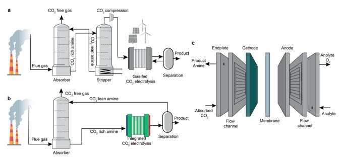
Fig. 1 Schematic illustration of (a) sequential CO2 capture and electrolysis based on gas-fed electrolysers, (b) an integrated route based on integrated electrolysers, and (c) cell configuration of a single cell of the integrated electrolysers.
