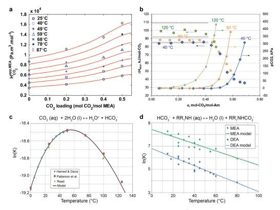
Fig. 3 The temperature effects on (a) Henry constant of  $CO_2$ , reproduced with permission, <sup>49</sup> copyright 2011, Elsevier. (b)  $CO_2$  partial pressure and heat of  $CO_2$  absorption for 30 wt% MEA aqueous solutions, reproduced with permission, <sup>50</sup> copyright 2014, Elsevier, (c) bicarbonate formation, and (d) carbamate formation for MEA and DEA aqueous solution. Reproduced with permission, <sup>51</sup> copyright 2017, Elsevier.
