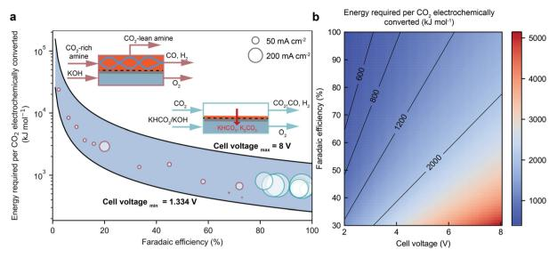
Fig. 6 (a) A comparison of the energy consumption, CO faradaic efficiency, and cell potentials over integrated and gas-fed CO<sub>2</sub> electrolysis. (b) The role of CO faradaic efficiency and cell voltage in determining the overall energy consumption of  $CO_2$  electrolysis to produce CO.
