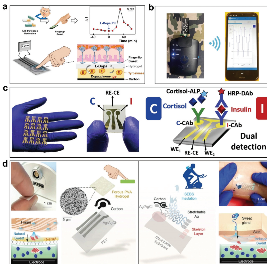
Fig. 6 Some sensors for other biomarkers. (a) The non-invasive sweat-based tracking of levodopa pharmacokinetic profiles following oral tablet administration. 161 This approach does not achieve wearability due to the special detection method used. This figure has been reproduced from ref. 161 with permission from Wiley-VCH GmbH; copyright: 2021. (b) A textile-based wearable solid-contact flexible fluoride sensor for the bio-detection of G-type nerve agents. 34 Based on the stretchability and breathability of flexible printed textiles and their potential for integration into clothing, this study achieves preliminary wearability. This figure has been reproduced from ref. 34 with permission from Elsevier B.V.; copyright: 2021. (c) Simultaneous cortisol/insulin microchip-based detection using dual enzyme tagging. 162 This device uses 0.76 mm-thick PETG (glycol-modified PET) as the substrate. However, PETG is non-stretchable and hard with a high elastic modulus and it does not achieve wearability. This figure has been reproduced from ref. 162 with permission from Elsevier B.V.; copyright: 2020. (d) A stretchable stress-free cortisol sensor based on touch. 163 The stretchable epidermal patch based on SEBS can adhere to skin. This figure has been reproduced from ref. 163 with permission from Wiley-VCH GmbH; copyright: 2021.
