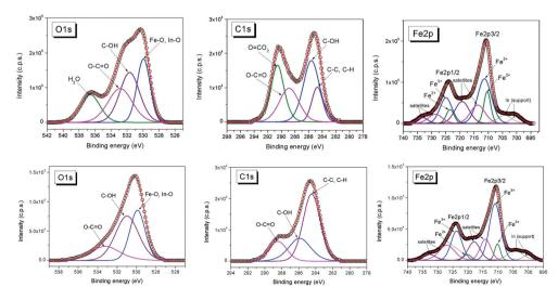
Fig. 6 O 1s, C 1s, and Fe 2p spectra of the (top row) original and (bottom row) acidified polygallate-containing magnetic nanoparticles (bottom row) aged for 4 weeks at pH  $\sim$  6.5 in 10 mM NaCl (reproduced from ref. 201 with permission from Am. Chem. Soc., copyright 2014).
