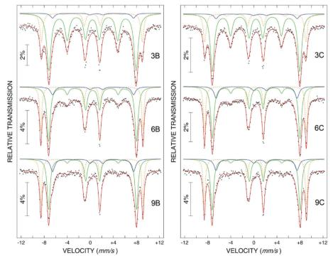
Fig. 10 Mössbauer spectra of Fe oxide nanoparticles collected at 4.2 K in 5 T applied field along the direction of  $\gamma$  rays, as corresponding to samples xB (without caping layer) and xC (with caping layer), where x=3 or 6 or 9, represents the mean diameter of nanoparticles in nm (reproduced from ref. 224 with permission from IOP Publishing, copyright 2012).
