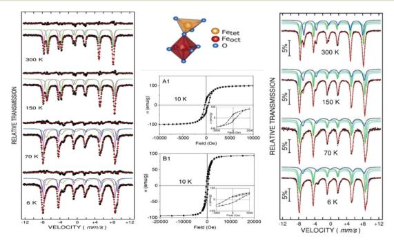
Fig. 9 Mössbauer spectra of hydrophilic Fe<sub>3</sub>O<sub>4</sub>-AZA (left) and MnFe<sub>2</sub>O<sub>4</sub>-AZA magnetic nanoparticles (right) at various temperatures in the magnetic frozen regime. In the middle there are the hysteresis loops collected at 10 K on Fe<sub>3</sub>O<sub>4</sub>-AZA (A1) and MnFe<sub>2</sub>O<sub>4</sub>-AZA (B1) (reproduced from ref. 221 with permission from Am. Chem. Soc., copyright 2021).
