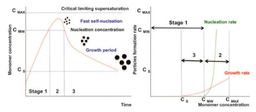
Fig. 3 Nucleation and growth model according to LaMer's theory (left) (reproduced from ref. 52 with permission from Am. Chem. Soc, copyright 1950). Comparison of nucleation and growth rates versus monomer concentration (right) (reproduced from ref. 54 with permission from Royal Soc. Chem., copyright 2018).
