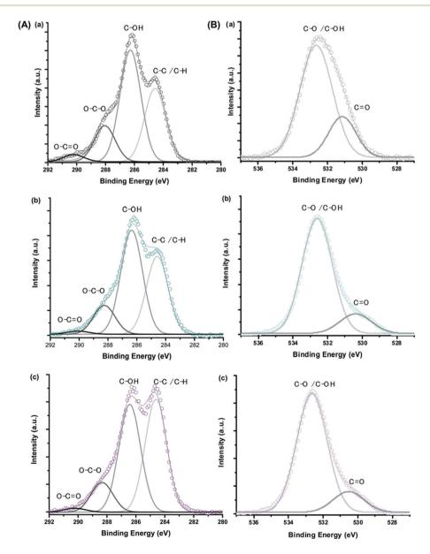
Fig. 8 XPS spectra of (A) C 1s and (B) O 1s regions obtained for (a) CMC ligand, (b) MION@CMC, and (c) Co10-MION@CMC (reproduced from ref. 212 with permission from Royal Soc. Chem., copyright 2021).
