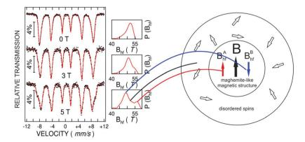
Fig. 11 Mössbauer spectra of Fe oxide nanoparticles of 6 nm mean size, collected at 3 K under increasing magnetic fields up to 5 T applied perpendicular on the direction of y rays and corresponding schematic representation of the spin structure of a nanoparticle. On the left side there are hysteresis loops of this sample, collected at different temperatures. Adapted with permission (reproduced from ref. 226 with permission from Nature, copyright 2020).
