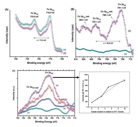
Fig. 7 XPS spectra of (A) Fe 2p and (B) Co 2p regions for (a) MION@CMC and (d) Co10-MION@CMC. (C) Spectra of the Co 2p<sub>3/2</sub> region for (a) MION@CMC, (b) Co3-MION@CMC, (c) Co5-MION@CMC, and (d) Co10-MION@CMC. Inset: evolution of intensity at the Co 2p<sub>3/2</sub> peak with increasing cobalt content (reproduced from ref. 212 with permission from Royal Soc. Chem., copyright 2021).
