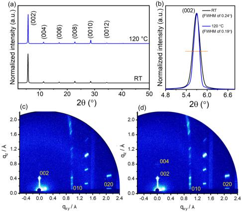
Fig. 3 (a) Out-of-plane XRD measured for  $(TEA)_2SnI_4$  thin films cast at RT and 120 °C. (b) FWHM analysis of the (002) peak. GIWAXS patterns for  $(TEA)_2SnI_4$  cast at (c) RT and (d) 120 °C (reflections are assigned by Miller indices).
