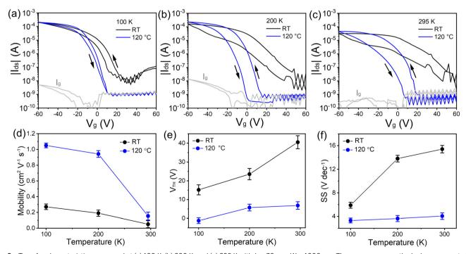
Fig. 5 Transfer characteristics measured at (a) 100 K, (b) 200 K, and (c) 295 K with  $L = 30 \mu m$ ,  $W = 1000 \mu m$ . The gray curves are the leakage currents ( $I_0$ ) between the source and gate electrodes in the 120 °C cast device. (d) Average hole charge carrier mobility, (e) threshold voltage and (f) subthreshold swing as a function of FET temperature. The error bars were calculated from 12 devices
