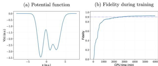
**Fig. 7** Learning performance of RL for (a) a potential that is difficult to solve with gradient-based quantum control methods. For this particular case, the NIC-CAGE algorithm fails to converge (with a transition probability of  $P < 10^{-28}$ ) after five hours of computation. In contrast, the DDQN-based reinforcement learning approach gives a higher fidelity and continues to improve as the algorithm runs longer, as shown in panel (b).
