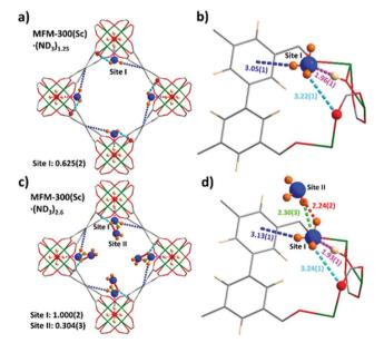
Fig. 2 Views of binding sites for ND<sub>3</sub> in MFM-300(Sc) determined by NPD at 10 K. The occupancy of each site has been converted into ND<sub>3</sub>/Sc for clarity. (a and c) Views along the c-axis showing packing of the guest molecules of ND<sub>3</sub> in MFM-300(Sc)·(ND<sub>3</sub>)<sub>1.25</sub> and MFM-300(Sc)·(ND<sub>3</sub>)<sub>2.6</sub>, respectively. (b and d) Detailed views of host-guest interactions between MFM-300(Sc) and adsorbed molecules of ND<sub>3</sub>.
