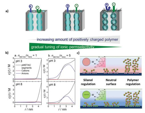
Fig. 4 (a) Schematic depiction of mesoporous silica thin films functionalized with PMETAC at various electrolyte density, (b) molar concentration of polymer segments, cations (K<sup>+</sup>) and anions (Cl<sup>-</sup>), as a function of the distance from the center of the pore, and (c) schematic depiction of the modified silica surface at acidic pH < 3 (upper figure) and alkaline pH > 7 (lower figure). Reprinted with permission from ref. 134 Copyright (2015), American Chemical Society
