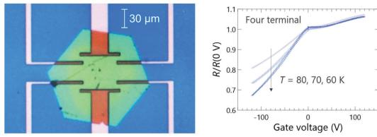
Fig. 9 Microscope image of the thin hexagonal crystal of  $[(S)-1]_9(Mo_6O_{19})_5$ . (CHBr<sub>3</sub>)<sub>2</sub> attached on the SiO<sub>2</sub>/Si substrate with pre-patterned gold electrodes (left). Gate voltage dependence of normalized resistance of the crystal at selected temperatures of 60 K, 70 K, and 80 K (right).
