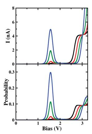
**Fig. 7** The upper panel shows the I-V characteristic of the boron-electrode connected junction at different gate voltages. The lower panel depicts the occupation probability of 7e-1st-es at 0.0 V <  $V_{\rm SD}$  < 3.5 V where different gate voltages have been applied. Black, red, green and blue solid lines represent the current (upper panel) and the probability (lower panel) with applied gate voltages of 0.15 V, 0.10 V, 0.05 V and 0 V, respectively.
