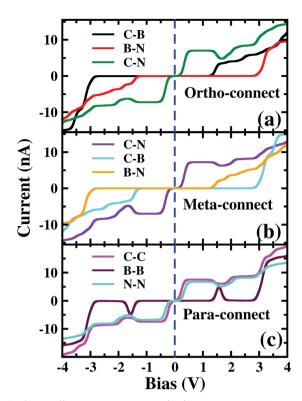
Fig. 1 Current (/)—source-drain voltage ( $V_{\rm SD}$ ) characteristics of a molecular device where the electrodes are connected in (a) ortho, (b) meta and (c) parapositions. The dashed blue line represents  $V_{\rm SD}=0.0$ . In the upper left corner, the atomic sites attached to the electrodes are stated. See Fig. S3 in the ESI† for the detailed geometry of the electrode-molecule-electrode configurations.
