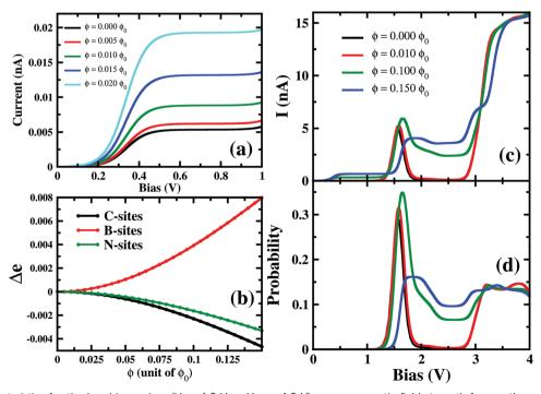
Fig. 5 (a) I-V characteristics for the low bias regime ( $V_{SD}$  of 0 V <  $V_{SD}$  < 1.0 V) versus magnetic field strength for paratha para-positioned boron connected device. (b) Charge density at the boron sites with varying magnetic field strength. (c) I-V characteristics and (d) occupation probabilities of 7e-1st-es at higher  $V_{SD}$ , for varying magnetic field strength.
