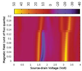
Fig. 6 The colour map shows differential conductance (dI/dV) as a function of  $V_{\rm SD}$  and applied perpendicular magnetic field  $(\phi)$  for the para-positioned boron connected device.
