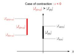
Fig. 7 Relationship between  $|J_{(0+x)}|$  and  $|J_{(0)}|$  in the case of bond contraction (x < 0).<sup>66</sup>
