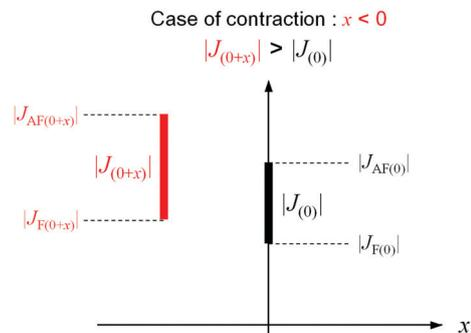
Fig. 7 Relationship between  $|J_{(0+x)}|$  and  $|J_{(0)}|$  in the case of bond contraction ( $x < 0$ ).<sup>66</sup>
