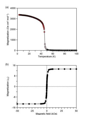
Fig. 2 Magnetic properties of MnW. (a) Magnetization vs. temperature plot at 20 Oe. (b) Magnetic hysteresis loop at 2 K.
