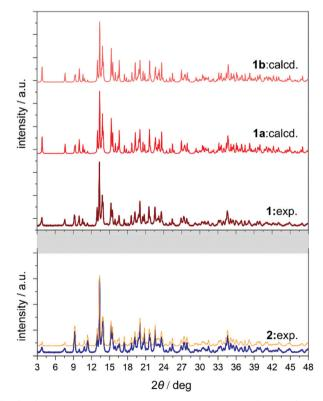
Fig. 2 Comparison of the experimental powder X-ray diffraction (P-XRD) pattern measured for **1** with the patterns for **1a** and **1b** calculated based on structural models obtained from the SC-XRD method (top), together with the experimental P-XRD pattern gathered for **2** which was compared with the pattern (orange line) obtained from the LeBail fitting procedure performed using EXPO 2014 software (bottom).
