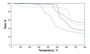
Fig. 4 TG traces collected under N<sub>2</sub> at a scan rate of 10° min<sup>-1</sup>: NppDI in black; NmpDI in magenta; NphDI in green; poly-NppDI in blue.
