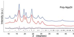
Fig. 1 Final Rietveld refinement plots, with difference plot and peak markers at the bottom. The observed and calculated curves (blue and red traces, respectively) have been vertically shifted for clarity.
