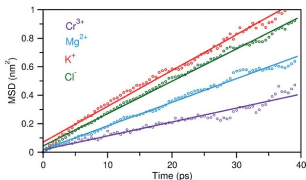
Fig. 6 Mean square displacement (MSD) of ions as a function of time, indicating faster dynamics in the order:  $\text{K}^+ > \text{Cl}^- > \text{Mg}^{2+} > \text{Cr}^{3+}$ . Dots represent the MSD data and solid lines are linear fits.
