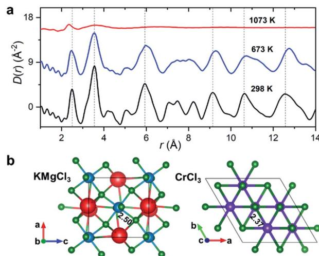
Fig. 1 Temperature-dependent PDF results. (a) X-ray reduced pair distribution functions,  $D(r)$ , for the  $\text{KCl-MgCl}_2$  salt mixture (50 : 50 mol%). (b)  $\text{KMgCl}_3$  ( $Pnma$ ) and  $\text{CrCl}_3$  ( $P3_12$ ) crystal structures with highlighted Mg–Cl and Cr–Cl average bond lengths in Å. Color scheme: K, red; Mg, blue; Cr, purple; Cl, green. Vertical dashed lines in (a) are guides to the eye.
