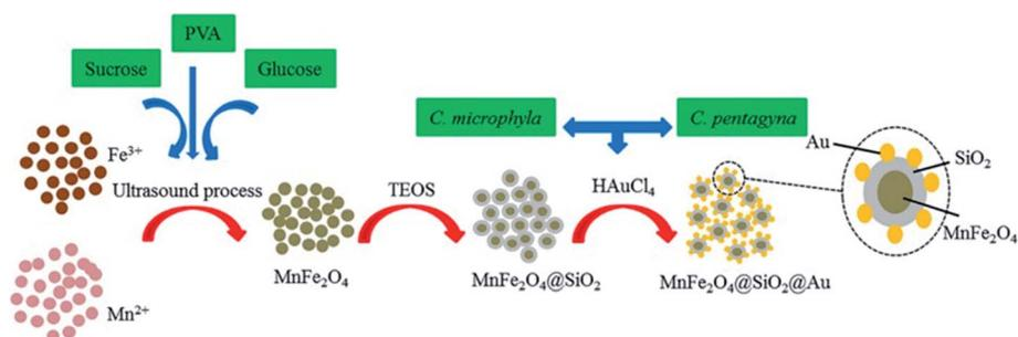
Fig. 6 Schematic illustration of nanocomposite preparation for antibacterial activity.<sup>60</sup>
