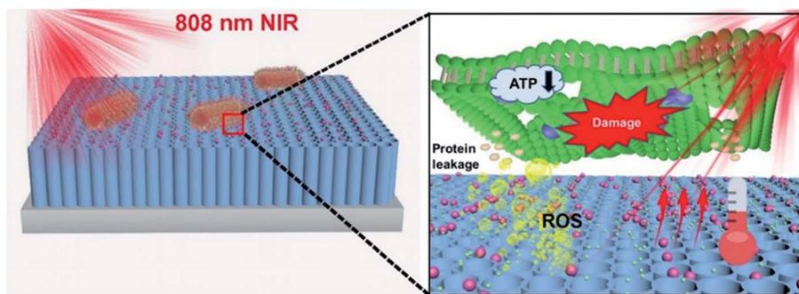
Fig. 7 A schematic image of the antibacterial mechanism of TNTs/Au/CDs under 808 nm NIR light irradiation within 15 min.<sup>65</sup>
