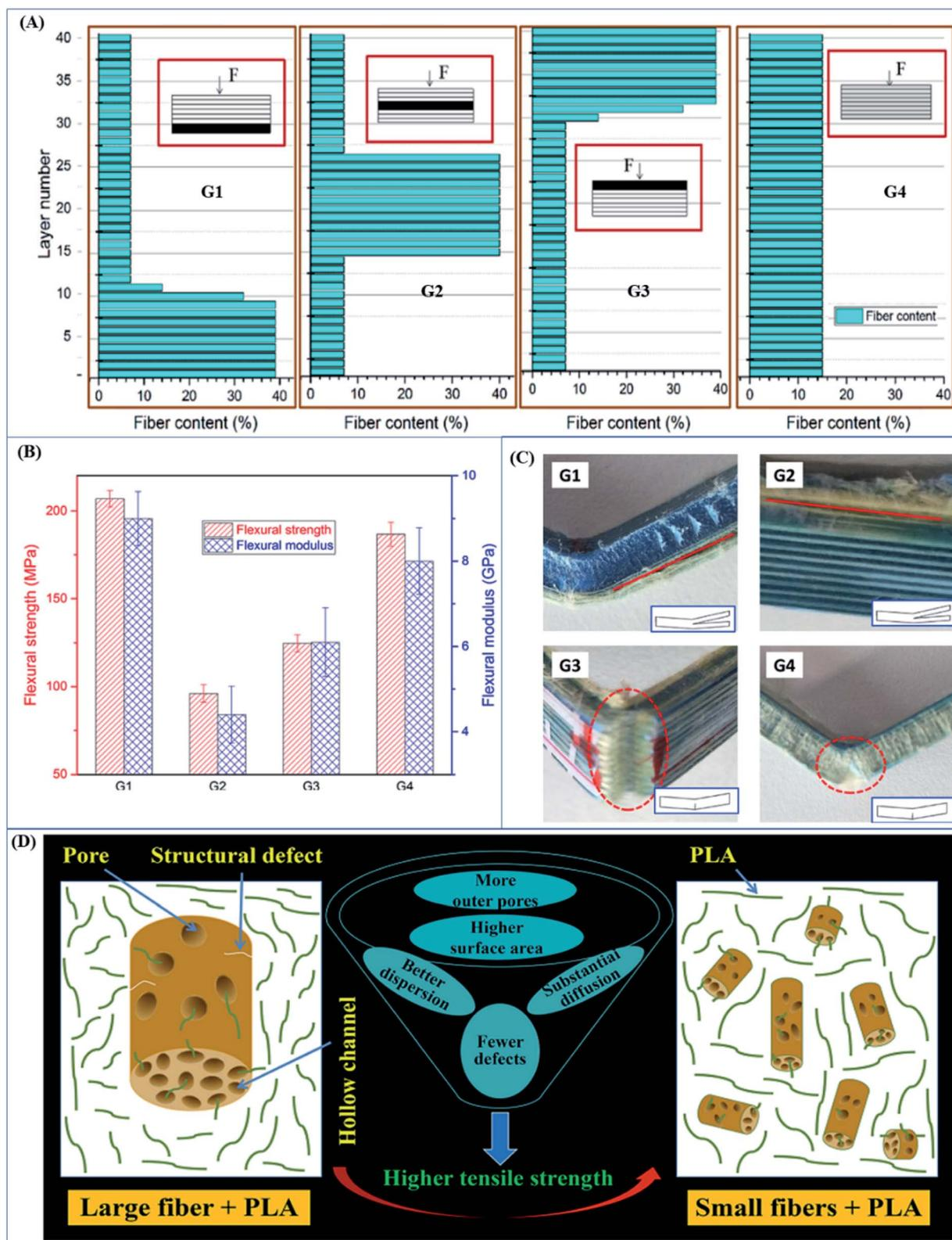
Fig. 11 (A) Illustration of CFRHCs fabricated using 3D printing, (B) effect of nonuniform fiber distribution on flexural properties and (C) failure mode of printed CFRHCs (adapted with permission).<sup>286</sup> Copyright 2020, Elsevier, License Number: 5143640554902. (D) Illustration of proposed dispersion of poplar fibers and PLA (adapted with permission).<sup>287</sup> Copyright 2019, American Chemical Society.
