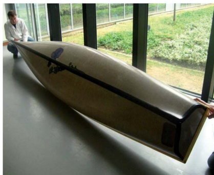
Fig. 2 Flax/PLA canoe manufactured during the NAVECOMAT project.
