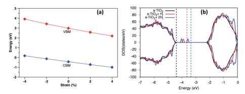
Fig. 4 (a) The calculated VBM and CBM of anatase using HSE06 under different biaxial strain. (b) The DOS of H doped  $a-TiO_2$  compared with pure  $a-TiO_2$ . The energy was aligned by the 1s state of O atom far away from the defect. The dashed line indicates the Fermi level of each system.
