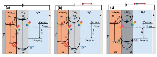
Fig. 1 Approximate energy band diagram and charge transfer mechanism of (a)  $Fe_2O_3-TiO_2$  photoanode without external applied anodic potential, (b)  $Fe_2O_3-TiO_2$  photoanode with external applied anodic potential and (c)  $Fe_2O_3-H:TiO_2$  photoanode with external applied anodic potential.
