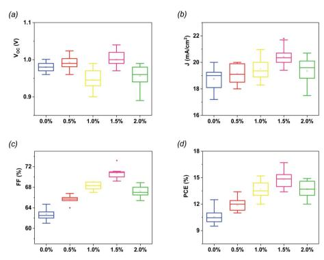
Fig. 2 Statistical histograms of photovoltaic parameters for different PSCs (a)  $V_{\rm oc}$ , (b)  $J_{\rm sc}$ , (c) FF and (d) PCE. Every box shows the parameter distribution of 20 devices.
