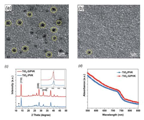
Fig. 3 (a) FESEM image of perovskite deposited on a pure  $TiO_2$  layer. (b) Perovskite on a G: $TiO_2$  layer. (c) XRD patterns of perovskites. The asterisk indicates the reflection of PbI<sub>2</sub>. Inset: zoomed-in view of the peak at 14° of the perovskites. (d) Absorption spectra of perovskite films deposited on pure and modified  $TiO_2$  layers.
