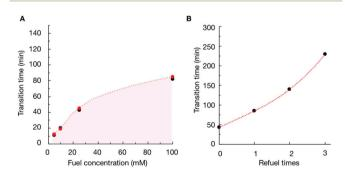
Fig. 3 (A) The time at which the anhydride to precursor ratio for P4 in the assembled state is around 55% as measured by HPLC and NMR (red markers) in combination with the time where fibers appear from confocal microscopy (black markers) as a function of fuel concentration. (B) Morphology transition time from colloids to fibers observed with confocal microscopy for P4 as a function of EDC refueling times. Refueling was done every 25 min up to 3 times with 25 mM of EDC.
