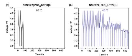
Fig. 1 Charge/discharge cycling of NMC622||Li cells with PEO-based SPE within a voltage range of 4.3-3.0 V and a specific current of 15 mA  $g^{-1}$  ( $\approx 0.1$ C) at (a) 60 °C and (b) 40 °C. The noisy voltage response during charge points to short circuits, whereby the onset of this failure tends to postpone at 40 °C.
