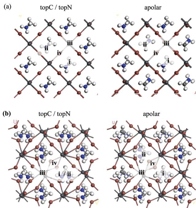
Fig. 3 Position of a fullerene C<sub>60</sub> on (a) cubic and (b) tetragonal MAPbI<sub>3</sub>(001) surfaces with MAI terminations for topC/topN and apolar geometries: (i) aboveN, (ii) aboveC, (iii) aboveI, and (iv) bridge. H, C, N, I, and Pb atoms are represented by the white, light grey, blue, brown, and dark grey spheres, respectively. H, C, N, I, and Pb atoms are represented by the white, light grey, blue, brown, and dark grey spheres, respectively.
